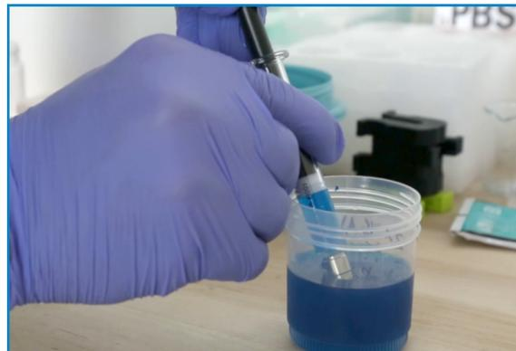
**5.5** Load syringe with sodium alginate
